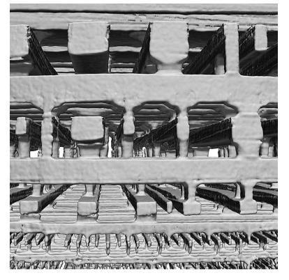
Our first technique, ptychographic X-ray computed tomography, was tested first on a portion of a 22-nanometer Intel processor constructing a detailed 3D image of the chip's interconnects.
