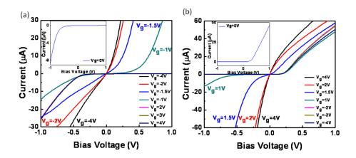
FIG. 2. *I*-*V*<sub>bias</sub> characteristics taken at different gate voltages ( $V_g$ ) of (a) graphene-Si (*p*-type) and (b) graphene-Si (*n*-type) devices. The inset figures show the *I*-*V* characteristics at  $V_g = 0$  V.
