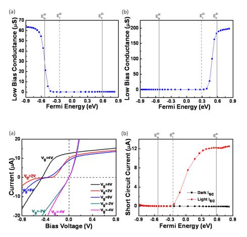
FIG. 3. Low bias conductance plotted as a function of graphene Fermi energy for (a) graphene-Si (*p*-type) and (b) graphene-Si (*n*-type) devices. The right and left solid vertical lines represent the conduction and valence bands of silicon, and the middle dashed line represents the Fermi energy of silicon.
