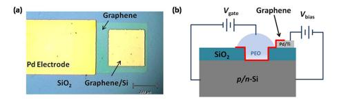
FIG. 1. (a) Optical microscope image of the graphene-on-silicon device before depositing the electrolyte top gate and (b) schematic diagram of the device structure.
