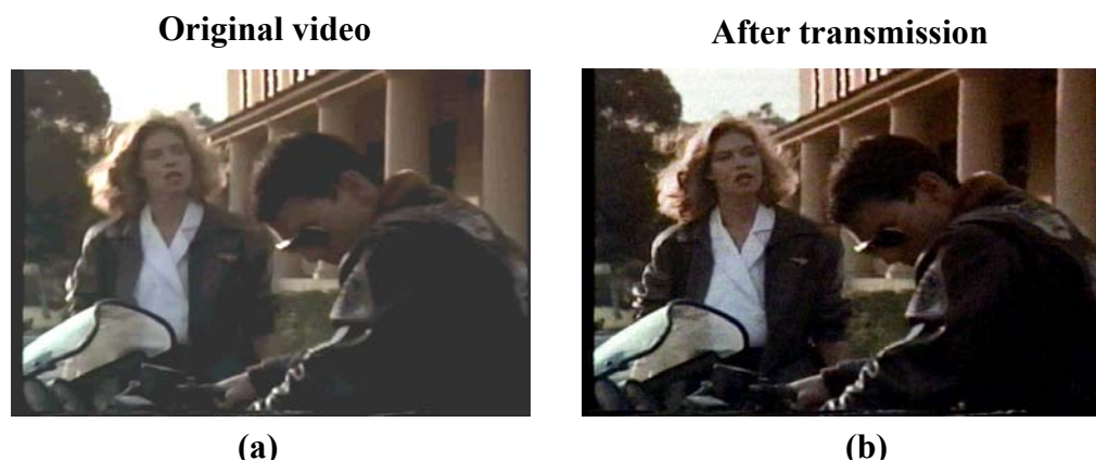
Figure 3.8 Demonstration of video transmission through microdisk based RF-optical link. (a) The original image. (b) The transmitted image.
