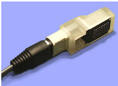
Figure 9 – Example of a prototype parallel fiber-optic transmitter module using VCSEL technology developed by Agilent [11]. The BGA for surface mount to a PCB and the 12 b -wide parallel fiber-optic push-pull connector are clearly visible. Today, such commercially available modules have a bandwidth density of 30 Gb/s/cm.
