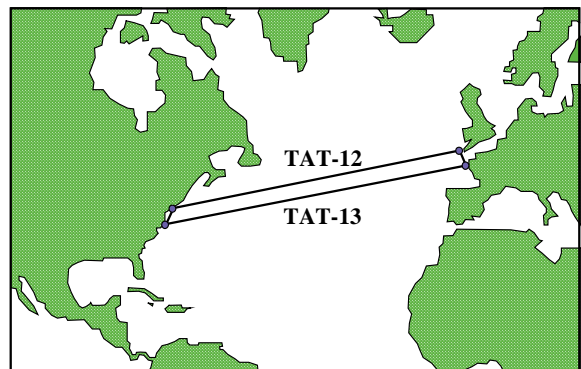
Fig. 6 – TAT 13/14 is a fiber-optic submarine cable WAN that connects the United States to Europe. Brought into service in 1995, it cost $0.75B and has an expected life of 25 years. It is a ring network consisting of two fiber pairs in each cable. Each pair transfers data at 5 Gb/s and the network has a capacity of 300,000 simultaneous voice channels. The total length of the ring is 14,000 km and there are fiber-optic amplifiers every 45 km.
