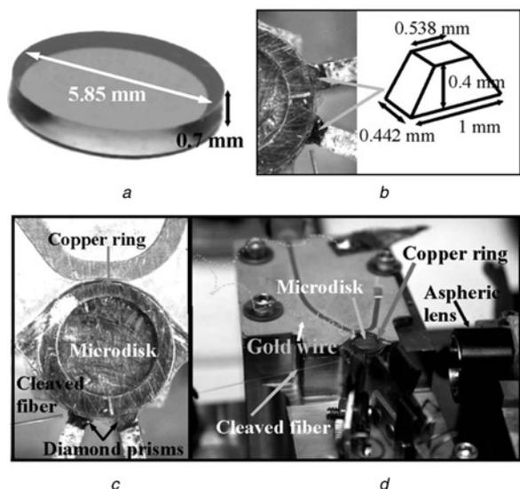
**Figure 1** Photograph of the microprisms and the microdisk
