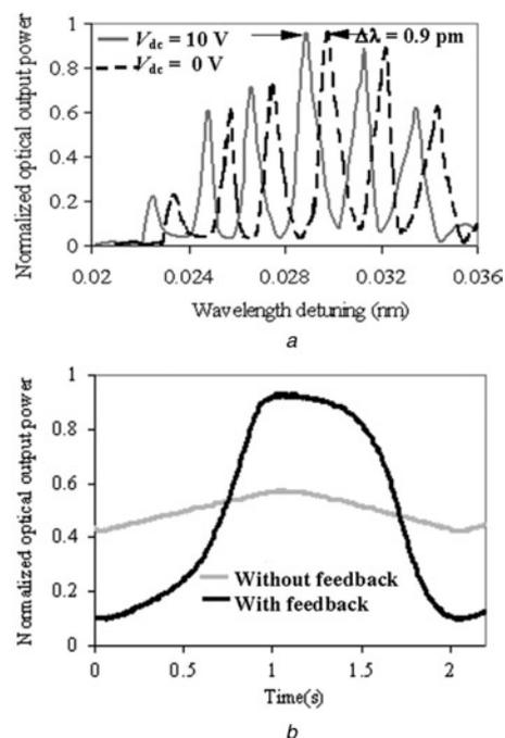
**Figure 3** Applied electric field changes the effective refractive index seen by light and shifts the spectral position of the high-*Q* TE whispering gallery resonances
