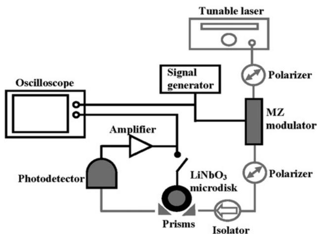
**Figure 2** Experimental arrangement to measure electro-optically induced nonlinearity
