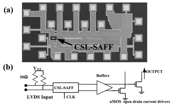
**Figure 4** (a) Die micrograph of the CSL SAFF test chip in 0.18  $\mu\text{m}$  CMOS with  $75 \times 75 \mu\text{m}^2$  bond pads. The location of the CSL-SAFF circuit is indicated by the white box and has an area of  $5 \times 40 \mu\text{m}^2$ . (b) Test circuit schematic diagram
