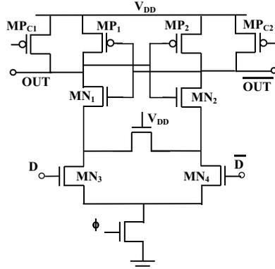
**Figure 1** Conventional voltage sense-amplifier (CVSA).
