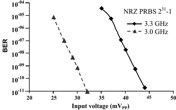
**Figure 5** Measured input sensitivity of the SAFF at 3.0 and 3.3 GHz. Sensitivity is better than 35 mV<sub>pp</sub> at 3.0 GHz (3.0 Gb/s) and better than 45 mV<sub>pp</sub> at 3.3 GHz (3.3 Gb/s) for a 10<sup>-11</sup> BER using NRZ PRBS 2<sup>31</sup>-1.
