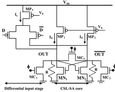
**Figure 2** Schematic of the current-steering logic sense-amplifier. Differential inputs are D and  $\bar{D}$ . Differential outputs are OUT and  $\bar{OUT}$ , and clock is  $\phi$ .
