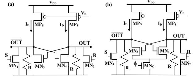
**Figure 3** (a) Current-steering SR Latch (b) Clocked current-steering SR Latch.
