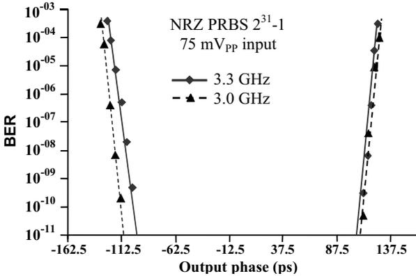
**Figure 6** Output phase margin of the test circuit at 3.0 and 3.3 GHz clock frequency for a NRZ PRBS 2<sup>31</sup>-1 input data pattern. The phase margin at 10<sup>-11</sup> BER is 200 ps (66% of the bit period) at 3.3 GHz (3.3 Gb/s).
